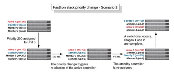
The following figure illustrates a hitless stacking switchover after the network administrator increases the priority value for two of the stack members.
