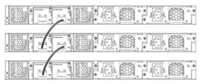
The following figure shows ICX 7450 units connected from 1 X 40-Gbps ports on the rear in a ring stack.
