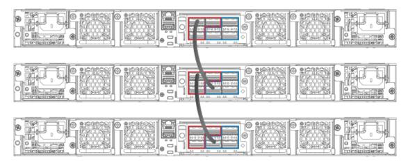
The following figures show ICX 7750 ring stacks from the front and rear panels. Default valid-stack-ports are located on the front panel, but they can be changed to the rear panel using the **stack-port** or **stack-trunk** command.
