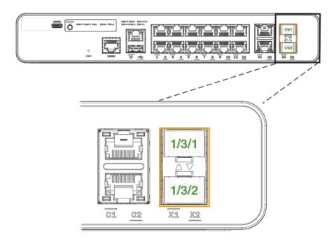
ICX 7150-24 and ICX 7150-24P devices have four stacking ports on the front panel.
