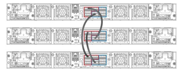
FIGURE 44 ICX 7750 Fully Populated Ring Stack from Rear Panel with Three-port Stacking Trunks
