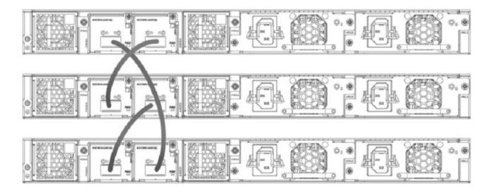
The following figure shows the ICX 7450 connected from the front in a ring using stacking trunks.
