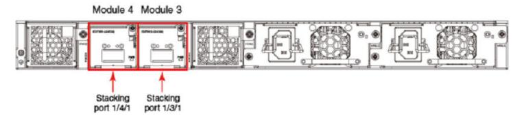
The following figure shows the 4X10GF module and port numbers.
