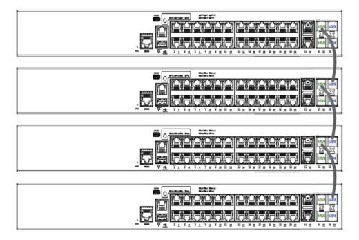
FIGURE 11 ICX 7150 24-port Stack Ring Topology
