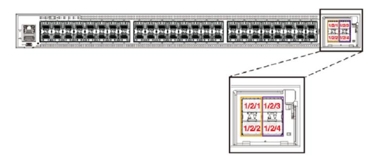
The following figure shows ICX 7450 units connected from 1 X 40-Gbps ports on the rear in a linear stack.
