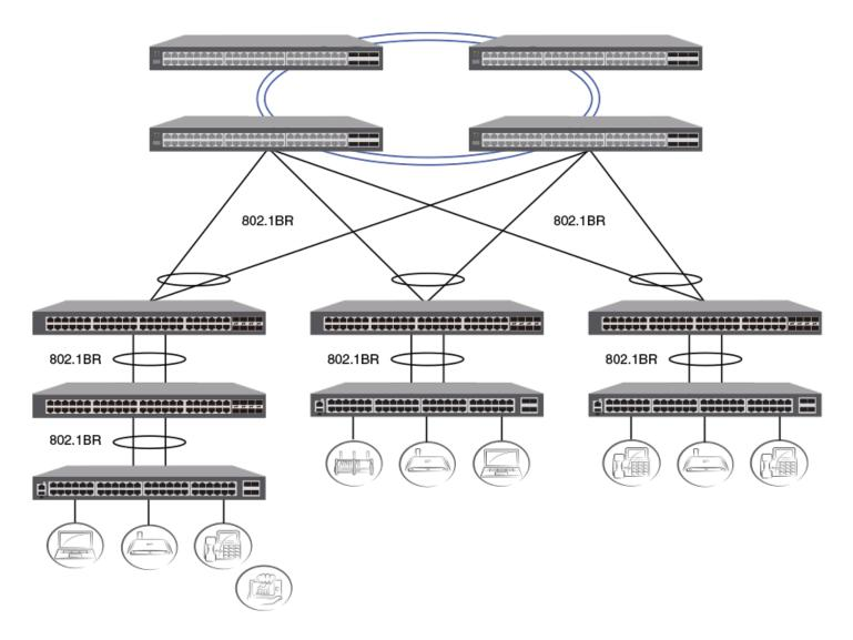
The following figure depicts three separate campuses, each with its own Campus Fabric domain, interconnected with a high-speed backbone.
