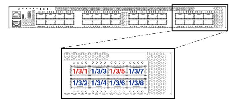
FIGURE 51 ICX 7850-48F/48FS Stacking Ports
