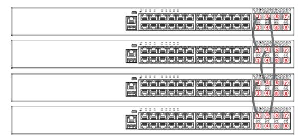
The following figure depicts a two-unit stack linear-topology trunk. All ICX 7250 models support this type of trunk, which improves redundancy and bandwidth. For more information, refer to Support for Two-unit Stack Linear-topology Trunks on page 33.
