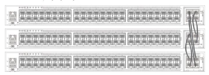
The following figure shows the ICX 7450 connected from the front in a linear stack using stacking trunks.
