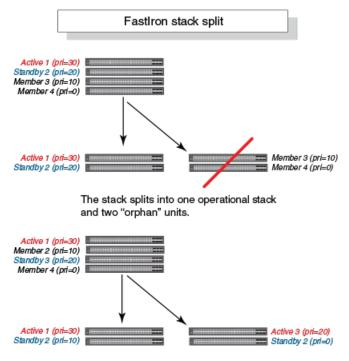
The stack splits into two operational stacks.
