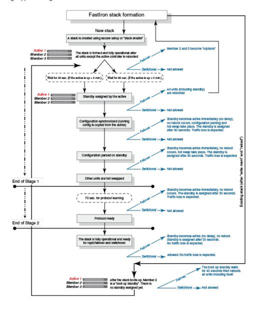
The following figure illustrates hitless stacking support during a stack merge.
