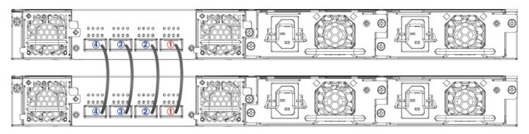
FIGURE 37 ICX 7650-48ZP Two-unit Stack Linear-topology Trunk (100 Gbps)
