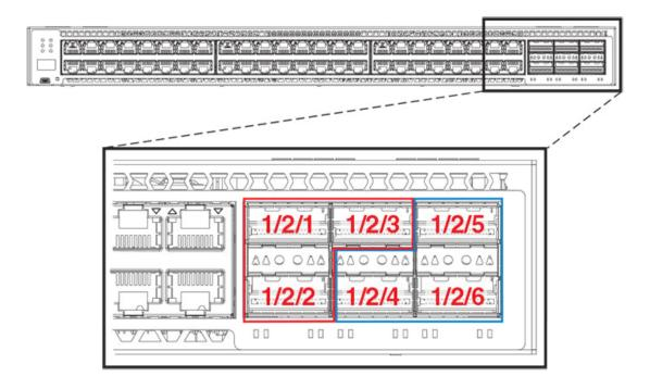
FIGURE 39 ICX 7750-26Q Front Panel Stacking Ports
