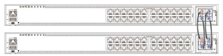
FIGURE 26 ICX 7450-24P Two-unit Stack with Linear-topology Trunk (Rear Panel)
