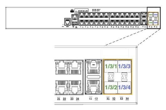
ICX 7150-48, ICX 7150-48P, ICX 7150-48PF, and ICX 7150-24F devices have four stacking ports in the same location on the front panel as ICX 7150 24-port models.
