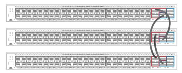
FIGURE 43 ICX 7750 Ring Stack from Rear Panel
