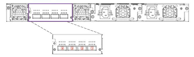
The rear module is fixed, and its ports can be configured for stacking or uplink. By default, the rear module supports 100-Gbps stacking on ports 1 and 2 (1/3/1 and 1/3/2). When 100-Gbps stacking is enabled, ports 3 and 4 are not used. Stacking trunks are not supported on 100-Gbps connections in a stack that contains more than two units. However, a 100-Gbps linear-topology trunk (ports 1/3/1 to 1/3/2) is supported in a two-unit stack.
