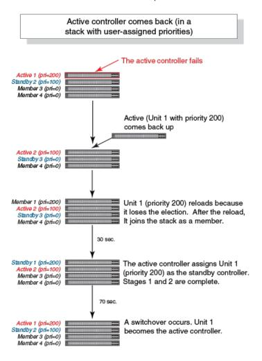
The following figure illustrates a hitless stacking switchover after the network administrator increases the priority value of the standby controller.
