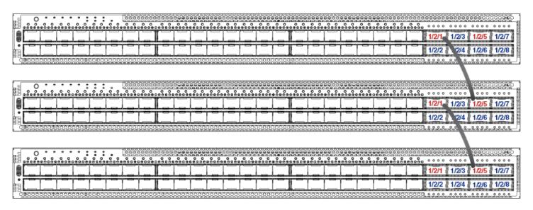
The following figure shows an ICX 7850-48F/48FS stack connected in a ring topology.
